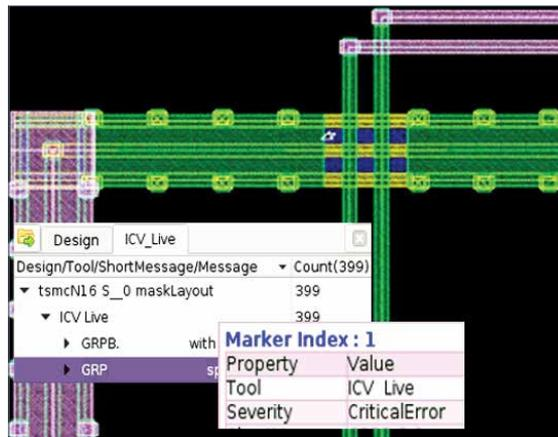
Figure 2: Live DRC checking for custom design flows
