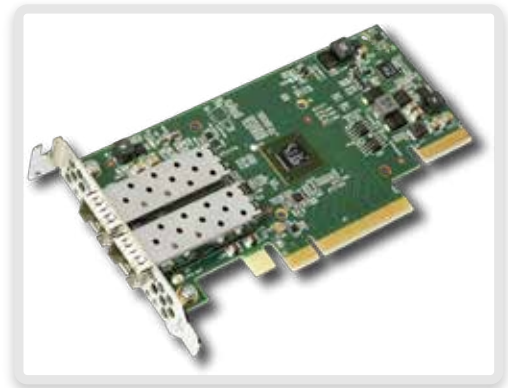
Figure 1: Solarflare Flareon 10/40G Network Controller with DesignWare IP for PCI Express 3.0
