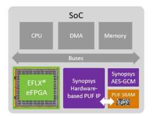
The system would power up just like any other eFPGA, but the AES-GCM will fetch the key from Synopsys Hardware-based PUF IP and decrypt the eFPGA configuration data before programming the eFPGA in the SoC. The configuration data can be stored in any non-volatile memory since it is protected by the key from the SRAM PUF. Not only will your supply chain be secure by using obfuscation, but the bitstream of the eFPGA can also no longer be altered, read, or copied to another device.
