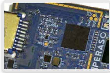
Figure 1: Peraso PRS4000 baseband processor
