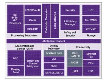
Figure 3: IP for connected vehicle and infotainment SoCs
