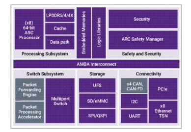
Figure 4: IP for gateway SoCs
