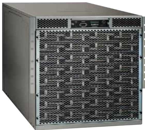
The SeaMicro SM10000-64 Server has 2,048 CPU cores per rack and provides the first server architecture that can support any CPU instruction set.
