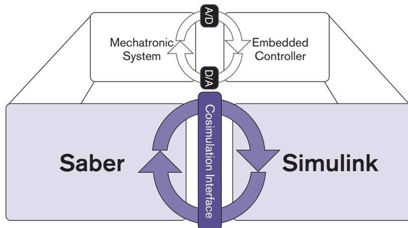
Figure 2. Saber-Simulink Co-simulation
