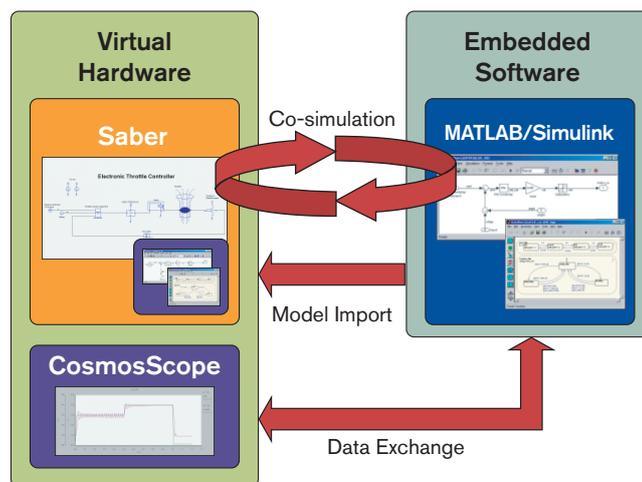
**Figure 5. Saber-MATLAB Integrations for Virtual HW/SW Co-verification**
