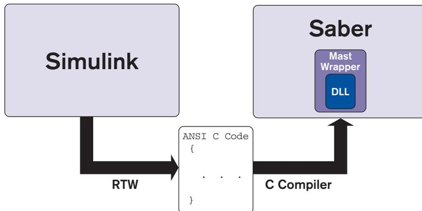
Figure 3. Simulink-to-Saber Model Import
