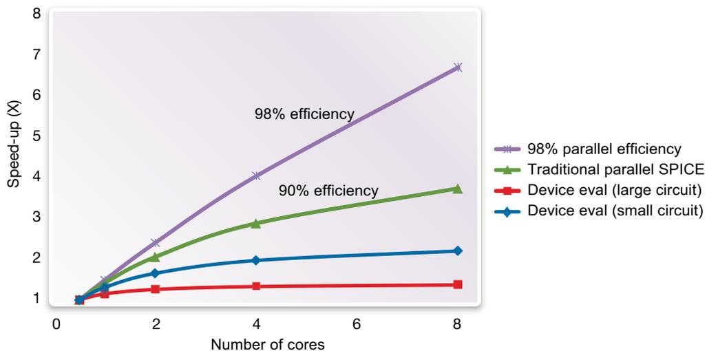
Figure 1: Theoretical limits of parallel SPICE simulation (Amdahl's Law)
