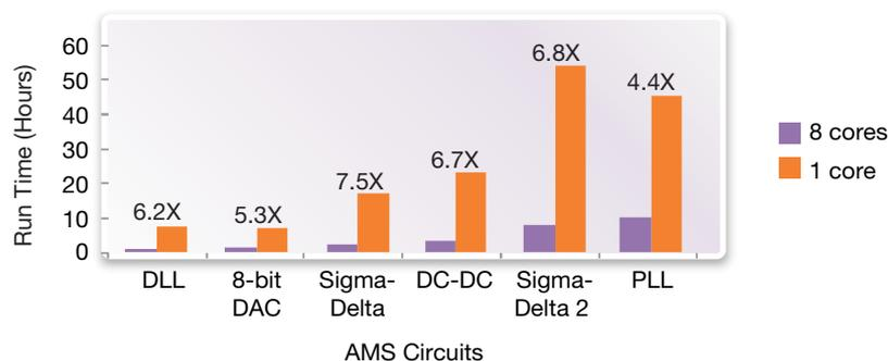
Figure 3: HSPICE multicore scaling on representative analog/mixed-signal circuits
