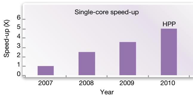
Figure 2: Single-core speed improvement in HSPICE
