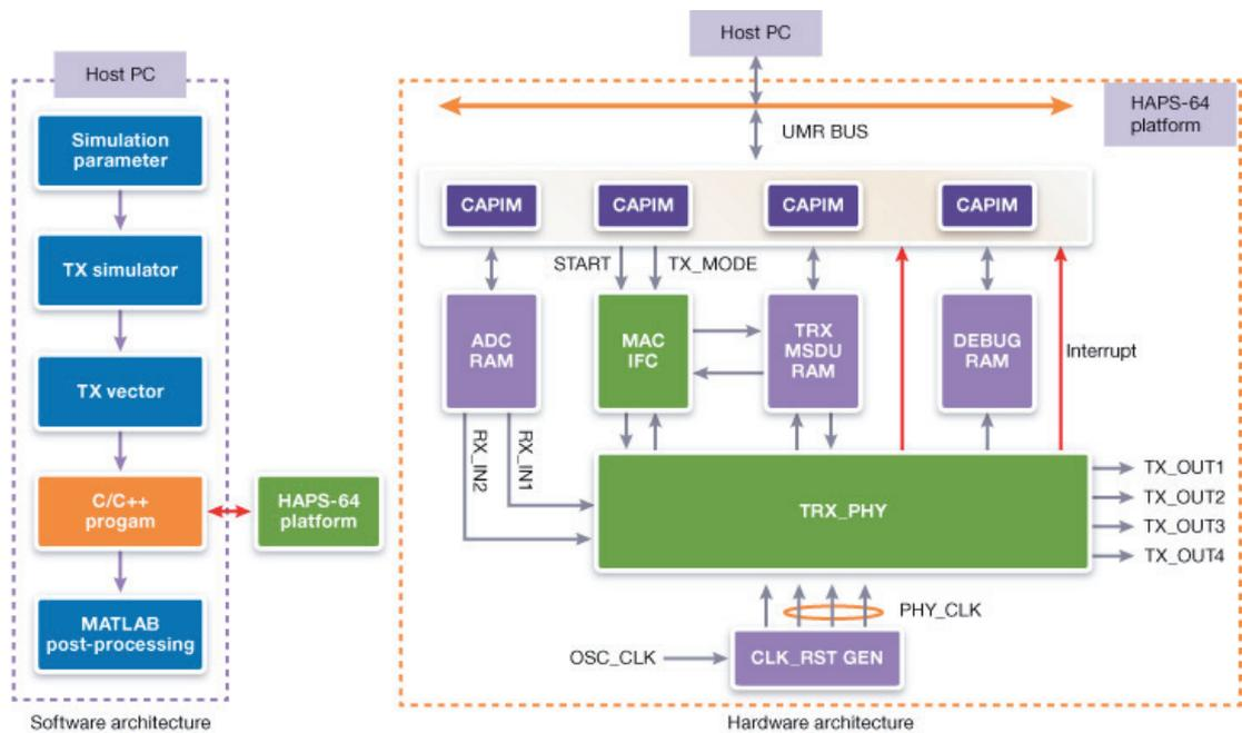
Figure 2: Kyutech HAPS-64 platform based WLAN transceiver demonstrator system architecture
