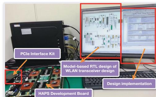
**Figure 1: Kyutech WLAN transceiver system demonstrator and validation platform using HAPS FPGA-based prototyping system**
