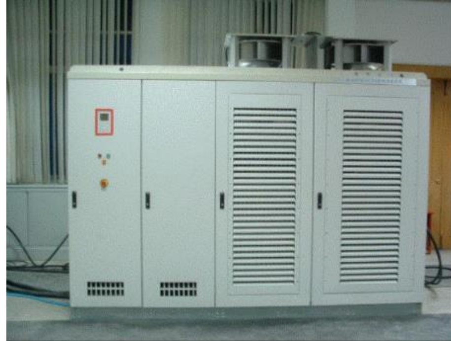
6000V/1.25MW IGCT based Three-Level NPC Inverter
