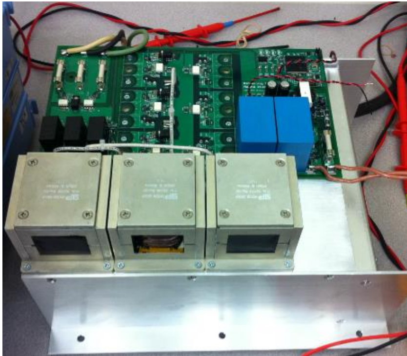
11kW/208VAC 97%-efficiency PFC
