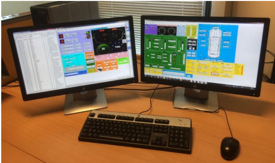
Fig. 5: D-EIPF running a full vehicle simulation
