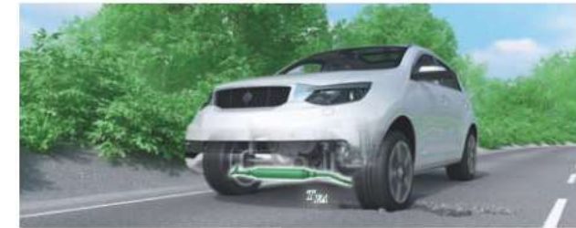
Decoupling: actuator torque front axle T_{FA} \hat{=} 0
