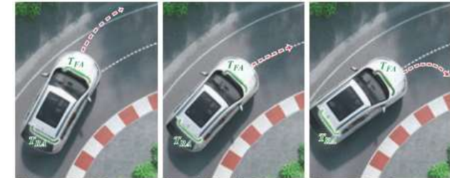
Understeer T_{FA} > T_{RA}
