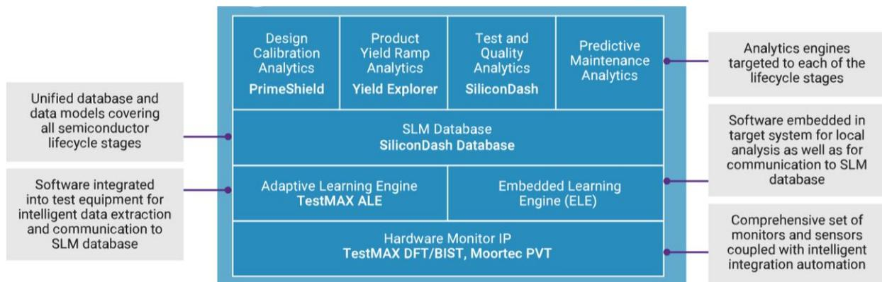
**The Synopsys SLM platform includes hardware monitors, learning engines, a product database and four analytic engines, three of which are currently available.**
