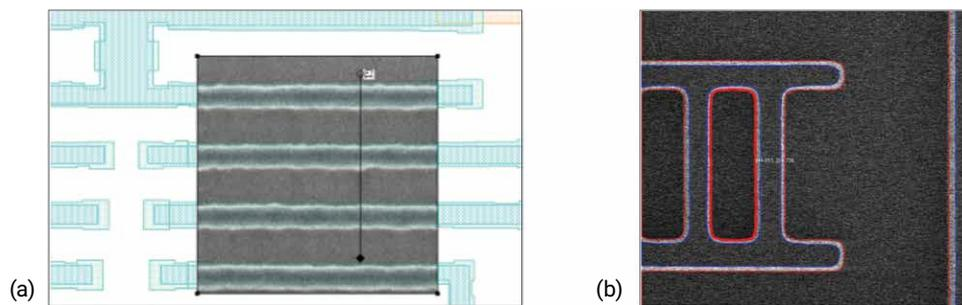
Figure 2: (a) Layout clip in Proteus WorkBench overlaid with SEM image through interface with S-Litho PWA Ultra
