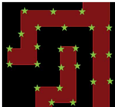
Flash: Discrete sampling in space domain at polygon edges.
