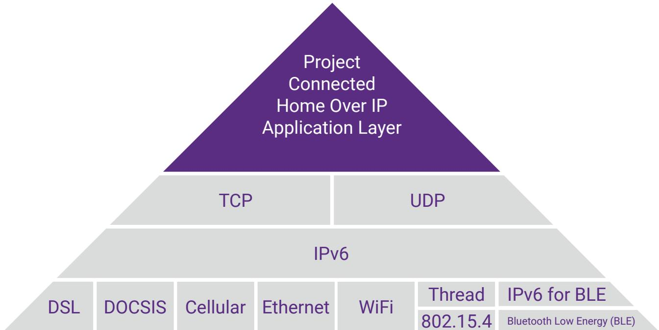
*Matter Technology Stack (Thread, Wi-Fi, and 802.15.4 directly relate to IoT and wireless communications)*
