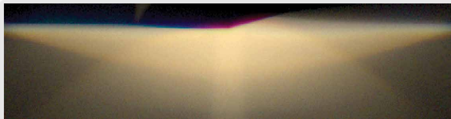
Figure 1. Results from a color simulation of a low beam lens headlamp (full view of a candela distribution).
