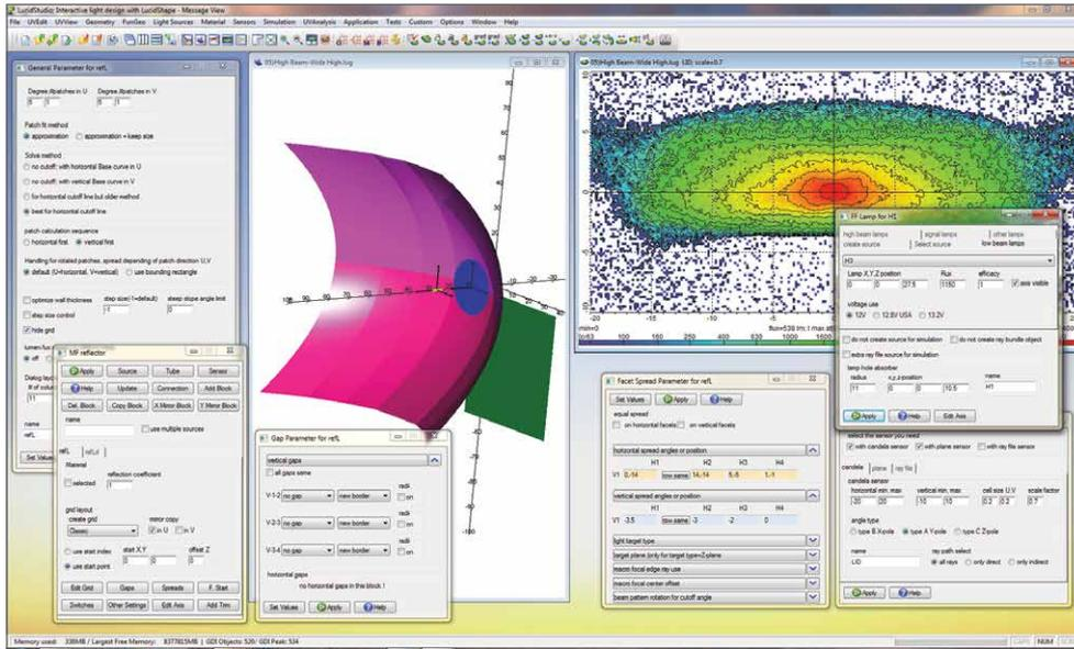
Figure 10: Automotive reflector design for a high beam function
