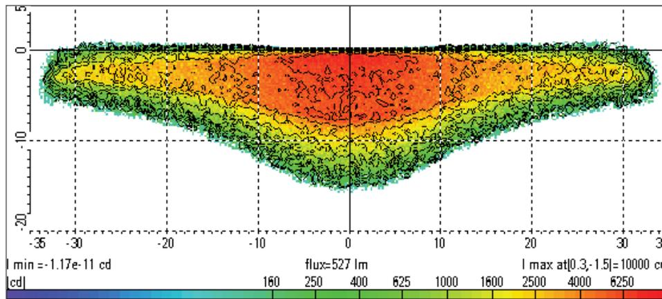
Figure 9: Beam pattern with sharp cutoff from freeform lens
