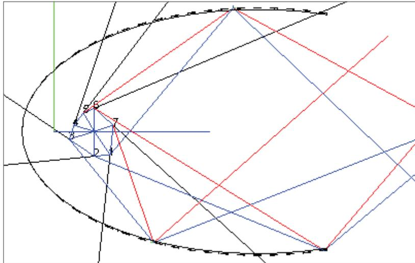
Figure 1: The concept of MF edge rays, shown on a reflector
