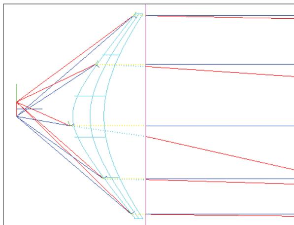
Figure 6: Freeform inner lens surface
