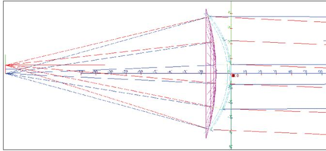
Figure 7: Freeform outer lens surface
