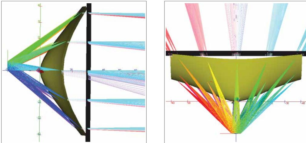
Figure 8: Freeform inner lens surface; vertical and horizontal spread
