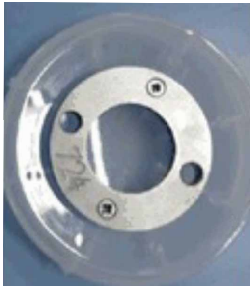
Figure 1: Picture of the sample (Window diameter = 20 mm ; Window Thickness = 1,5 mm)
