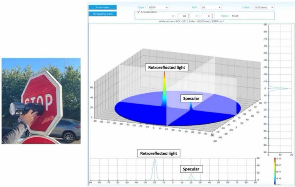
Measurement of the white area of a STOP sign for AOI=20° with Green light
