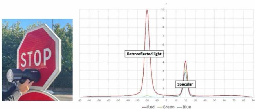
BxDF cross section of the red area measurement for AOI=20° with Red, Green and Blue light
