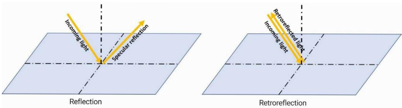
Figure 1: Illustration of reflection and retroreflection
