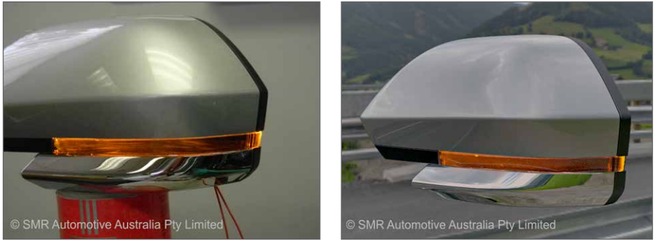
Figure 1: Side mirror indicator; Left: Photograph, Right: Photorealistic simulation with LucidShape's visualize module
