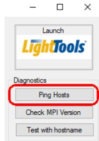
This button initiates a test communication to each host using the Windows ping command and displays the communication time in the Ping (ms) column of the table.
