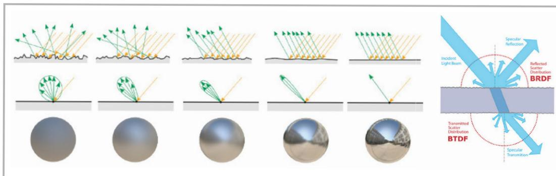
By definition transmittance and reflectance values from a sample can be measured from BSDF. It is the integral of it on the complete sphere.
