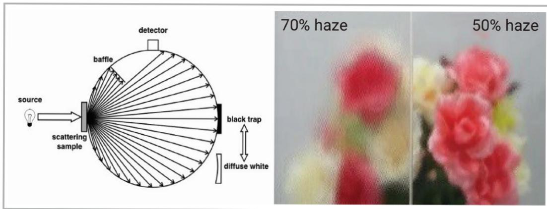
BSDF is a goniophotometric measurement of the light scattering off and through the surface of a material.
