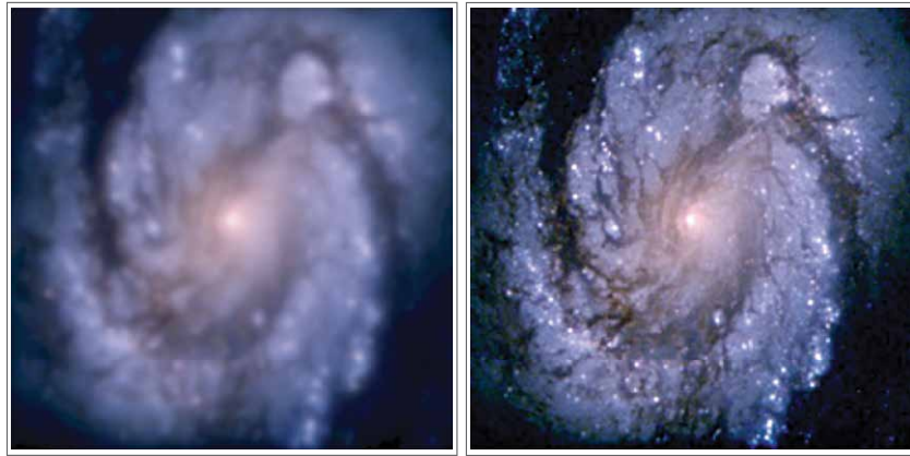
Figure 4a: Simulation with actual conic constant and 4b: Simulation with desired conic constant
