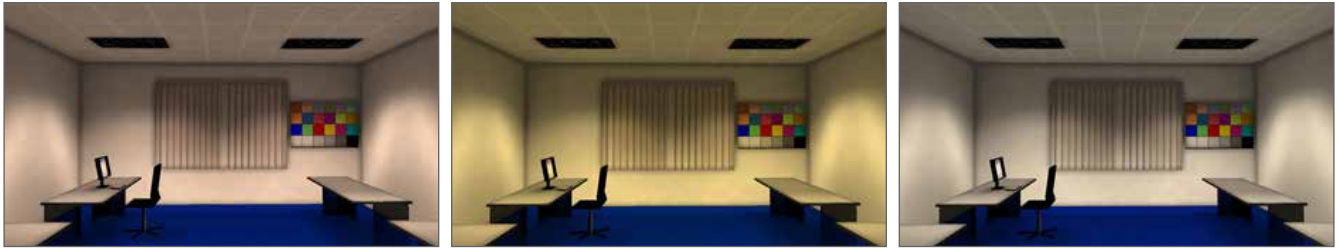
Figure 3: Comparison of photorealistic renderings of an office scene using three spectra: (a) 5000K black body spectrum, (b) 5000K Fluorescent spectrum of the lamps used to design the fixtures, and (c) 5000K white phosphor LED
