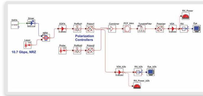
Figure 2. PCF simulation setup schematics in OptSim
