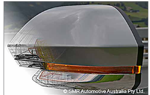
Figure 1: Wireframe and photorealistic image of a side mirror with LucidShape's Visualize Module
