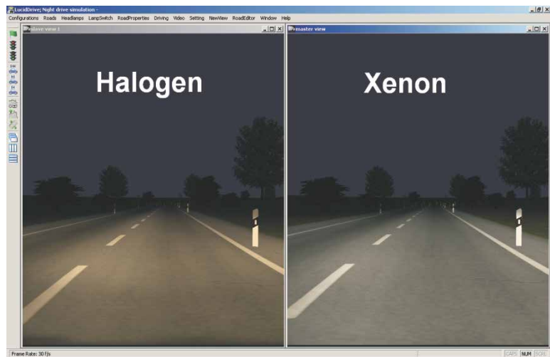
Figure 2. Halogen vs. Xenon headlamp simulation
