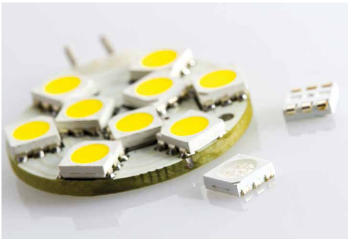
Illumination design: LED sources
