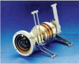
Wide-angle lightning imaging lens designed by our engineers and fabricated by Kaiser Electro-Optics, Inc. for NASA (photo courtesy of Kaiser Electro-Optics, Inc.)
