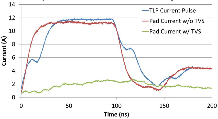
Measurements show actual current through the IC pad with  $\approx 1/3~\Omega$  resistance between IO and Vss
