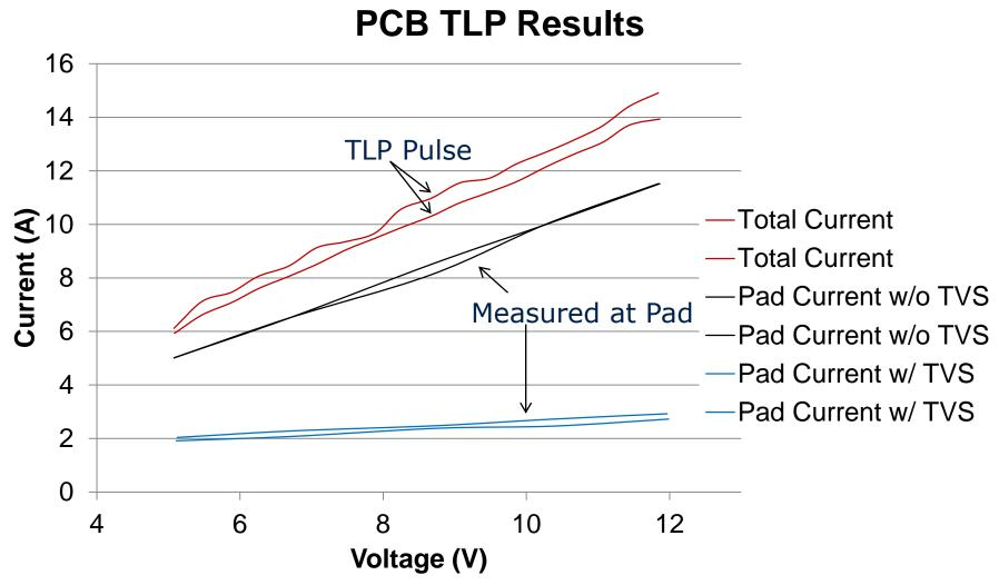
TVS turns on and reduces current at the pad by 9A
