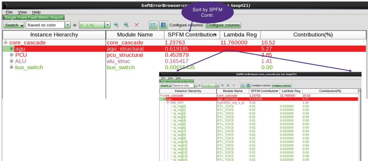
Figure 2: SPFM Browser identifies the blocks in the design with the highest probability causing functional safety failure
