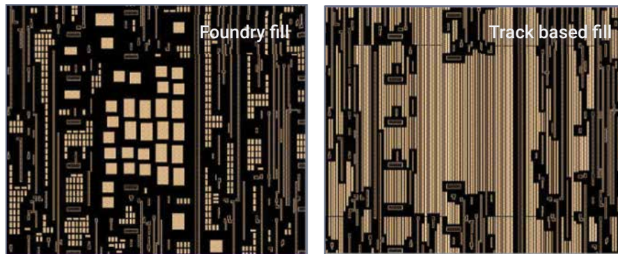
Figure 6: IC Validator In-Design metal fill color aware metal fill, optimized for density and foundry requirements
