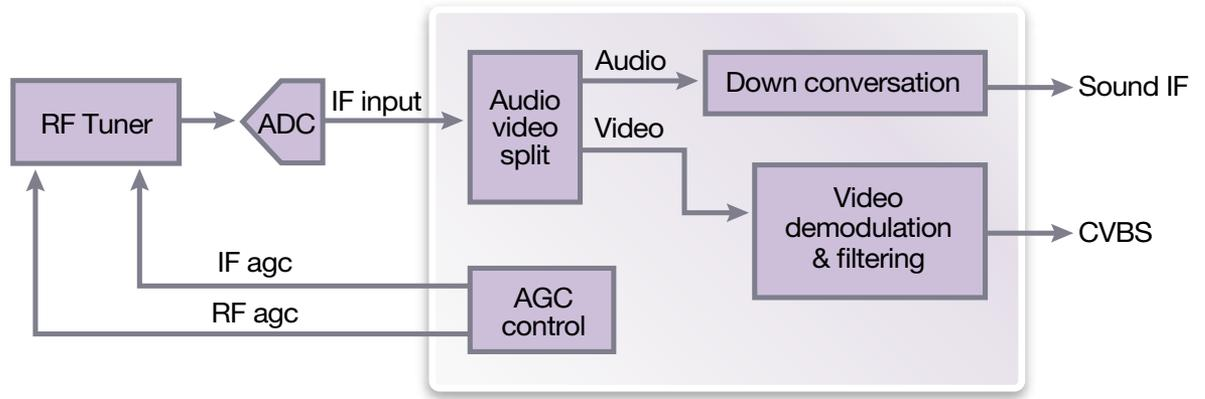
Figure 1: Digital Intermediate Frequency (DIF)
