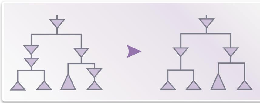
Figure 6. Only sinks that are timing critical need to be balanced
