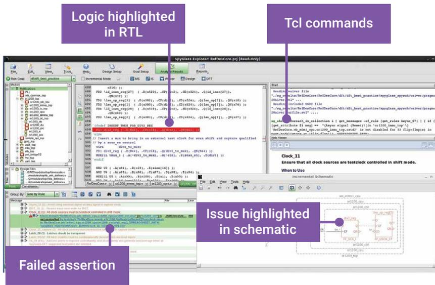
Figure 2: Integrated debug environment enables cross-probing among views to easily diagnose testability issues.
