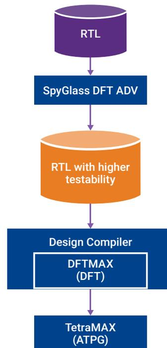
Figure 1: SpyGlass DFT ADV addresses testability issues early in the design flow.
