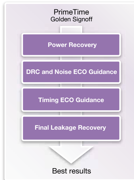
Figure 4. PrimeTime ECO Power Recovery Flow
