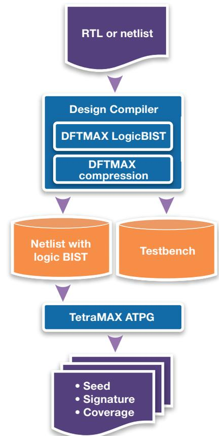
**Figure 1: Synopsys synthesis-based logic BIST flow**
