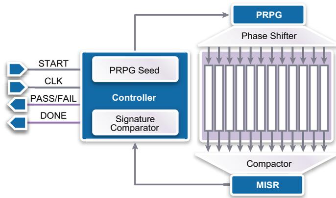
Figure 2: DFTMAX LogicBIST architecture
