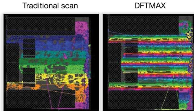
**Figure 4. These screen captures show DFTMAX results without the routing congestion associated with standard scan**
