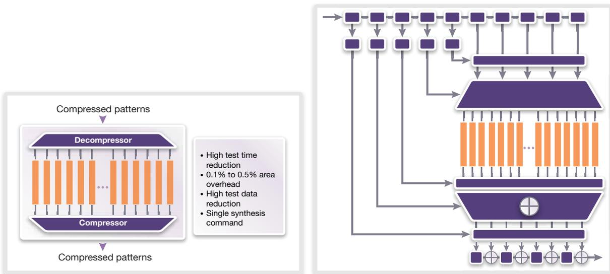
Figure 2a. (left) DFTMAX, Figure 2b. (right) DFTMAX Ultra minimizes the required number of scan I/O for pin-limited testing
