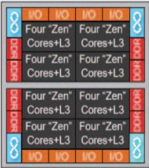
Monolithic 32-core Chip 777mm 2 total area 1.0x Cost
