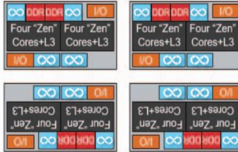
4 x 8-core Chiplet, 213mm 2 per chiplet 852mm 2 total area (+9.7%) 0.59x Cost
