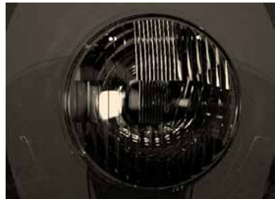
Figure 4: Simulation of lit appearance with a virtual Luminance Camera
